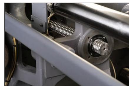
Ball screws are designed to push heavier loads, spreading the load across a much larger surface area than conventional ball screws.
