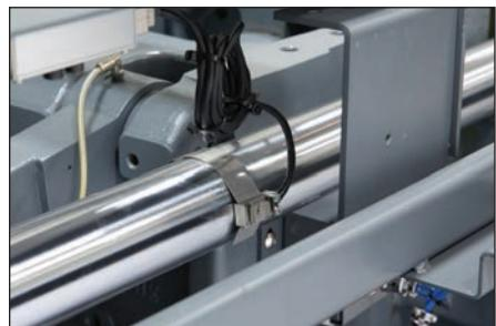
Strain gauge adjusts tonnage automatically and on the fly during the cycle. This ensures accurate tonnage at all times.
